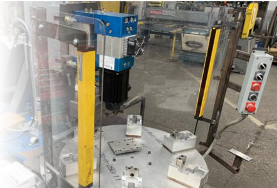
A Kyntronics SMART Hydraulic Actuator (SHA) model S12C32-07 rated for up to 20,000 lbf (89kN) with 4-inch (102 mm) stroke was selected to cover the wide force and position range needed to press various product sizes and types.
