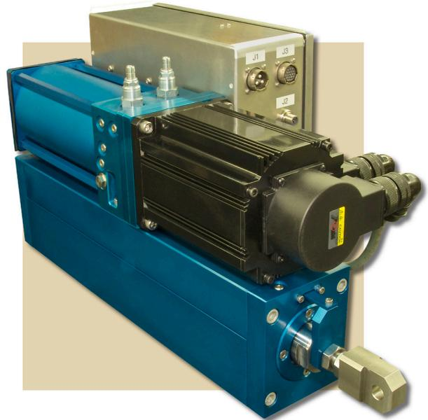
**The Electro Hydraulic Actuator from Kyntronics contains a complete hydraulic system within a self-contained modular assembly. Closed-loop force and position control are provided by built-in transducers, and power is transmitted by a variable-speed motor and control driving a hydraulic gear pump.**
