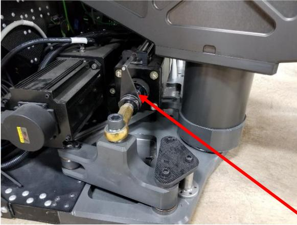
Coxa actuator installed on the vehicle. This actuator is responsible for rotating the leg around its vertical axis (analogous to the hipjoint). A linkage was used in order to transform the 6" stroke of the actuator into 180 degrees of rotation
