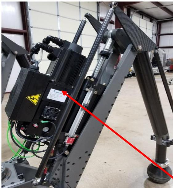
The tibia actuator is the last active joint in the leg. The tarsus joint (which is attached to the foot) is driven by a bellcrank mechanism that keeps the foot perpendicular to the ground without requiring active control. The position sensor can be seen on the side of the actuator. This sensor provides position feedback on the rod position of the actuator, which is used to calculate the overall pose of the leg
