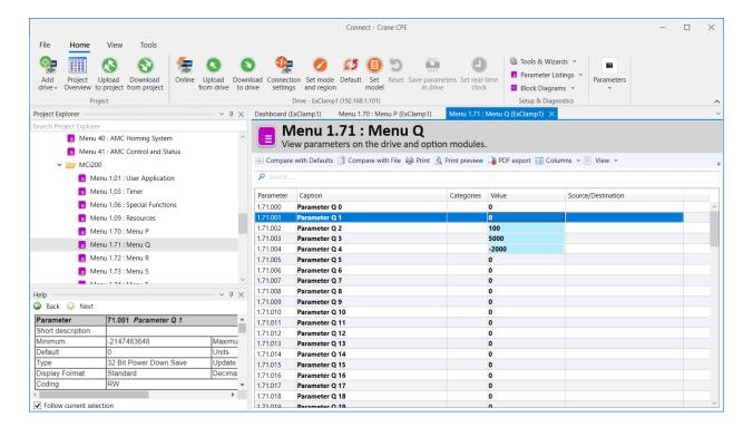
Here is where the non-drive menu items are hiding. All menu items have three fields, such as 1.71.003. The first field specifies the device, the second field is the menu, and the third is the specific parameter. The drive itself is device zero, and the option modules use their slot number.
