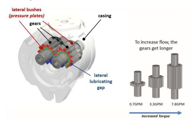
The size of the pump will determine the speed of the rod and will affect the amount of motor torque needed to reach the desired pressure and force. A smaller pump translates to slower rod speed, but then needs less motor torque to reach a given force. Higher flow (increased speeds) requires higher torques.
