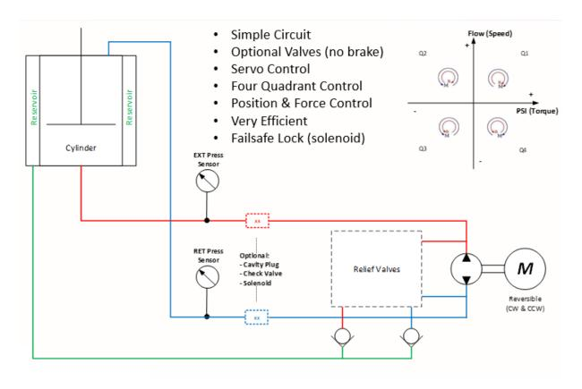
The Extend / Retract speeds & force (ratios) will be different with single-ended rod (usually provided). The retract direction has a smaller area (vs. the extend) which equates to a lower force and higher speed.
