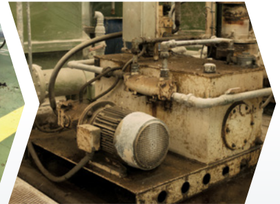
Constantly Running HPU Wastes Energy
