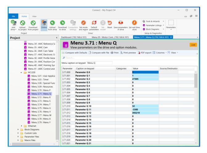
Here is where the non-drive menu items are hiding. All menu items have three fields, such as 3.71.003. The first field specifies the device, the second field is the menu, and the third is the specific parameter. The drive itself is device zero, and the option modules use their slot number.
