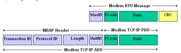
This shows how Modbus packets are incorporated into Modbus TCP. Use standard Modbus TCP Ethernet port 502.
